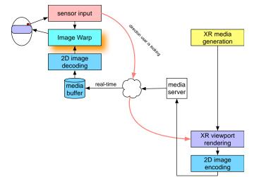
Figure 6: Split Rendering with Asynchronous Time Warping (ATW) Correction
