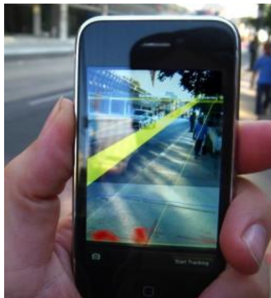
Figure 3: Example of video see-through AR on a smartphone. Source: Wikipedia
