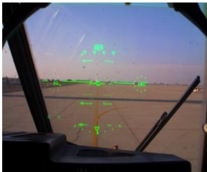
Figure 5: Example of an optical see-through display for an aircraft windshield. Source Wikipedia
